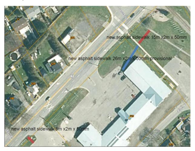
**Replacement of Existing Asphalt Sidewalk** – requires saw cutting or equivalent to existing asphalt driveways to create a clean butt joint for tie-in of new asphalt sidewalk. Additional of granular A as required for leveling and compaction of subsurface prior to installation of new asphalt sidewalk. Install a 1.5m wide 50mm HL3 asphalt sidewalk per OPSS specification.
