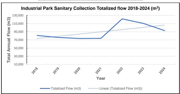
Totalized flow into the Prescott WPCP steadily declined from 2018 through 2021. Flow increased between 2021 to 2023 due to increased industrial usage and above average precipitation. Totalized flow in 2024 decreased by approximately 16% compared to 2023.
