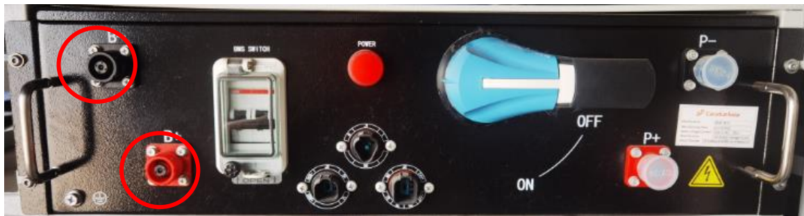
Figure 10. SolBank3.0 Battery Pack. Battery terminal and MSD indicated by red circle.
